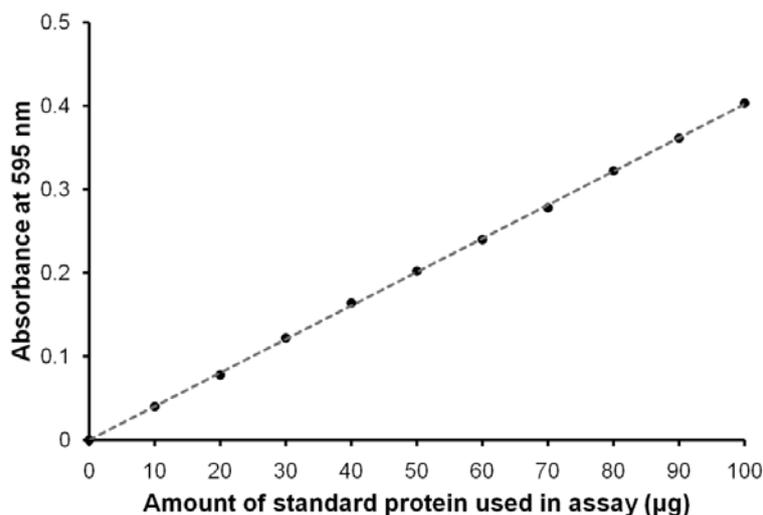
Figure 5.2: Plot of absorbance at 595 nm against the amount of protein
