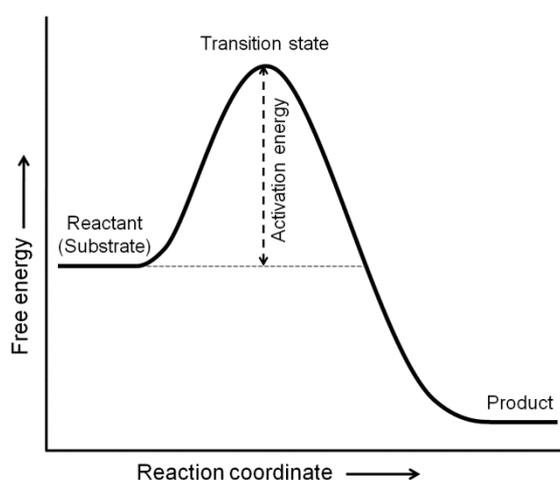
Figure 12.1: A diagrammatic representation of free energies of reactant, transition state, and the product
