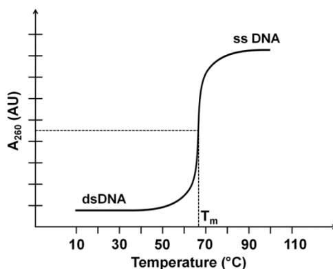
Figure 7.2: A typical DNA melting curve; the temperature at which half of the DNA is denatured is termed as the melting temperature ( $T_m$ ).
