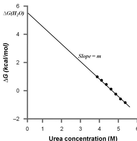
**Figure 8.3:  $\Delta G$  as a function of denaturant (urea) concentration. Intercept at  $\Delta G$  gives the stability of the protein,  $\Delta G(H_2O)$ .**
