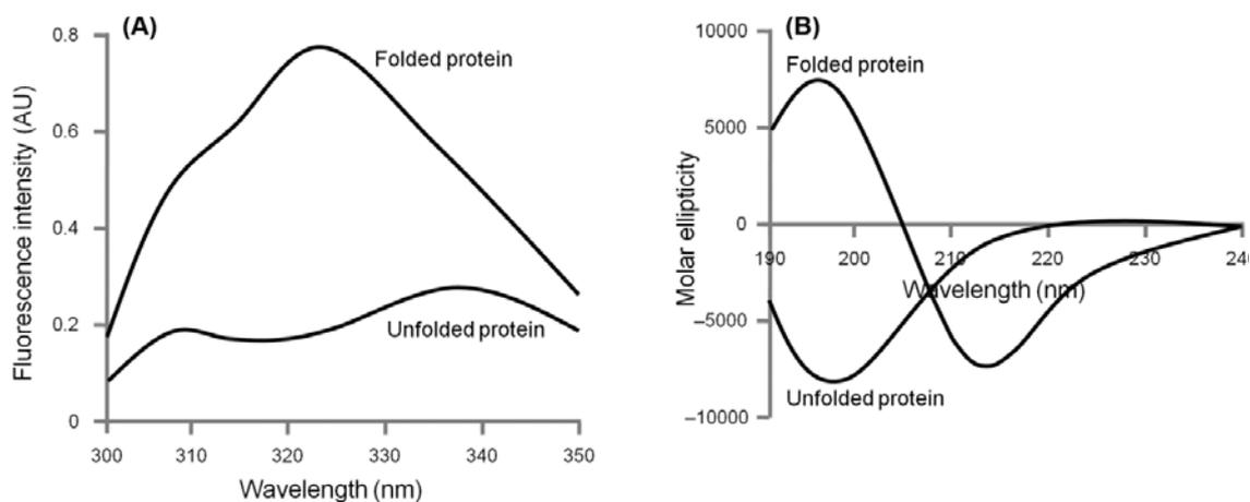
**Figure 8.1: Fluorescence and circular dichroism spectra of a hypothetical protein in folded and unfolded state**
