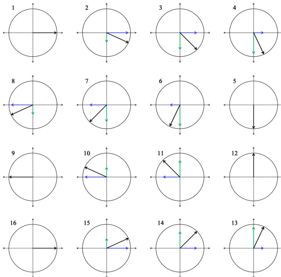
**Figure 9.1** Generation of circularly polarized light through superposition of two plane polarized waves (blue and green), polarized in two perpendicular planes and out of phase by  $90^\circ$ . Only electric field vectors are shown here for clarity.
