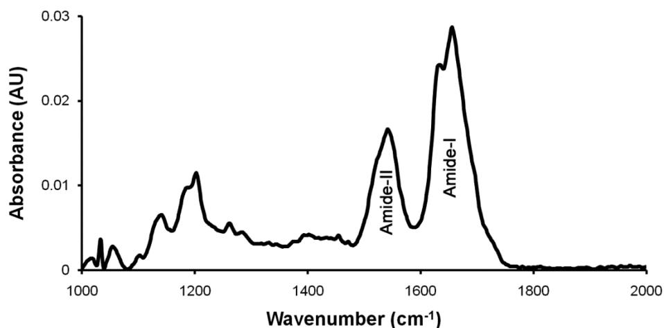
Figure 11.2: An infrared spectrum of a polypeptide
