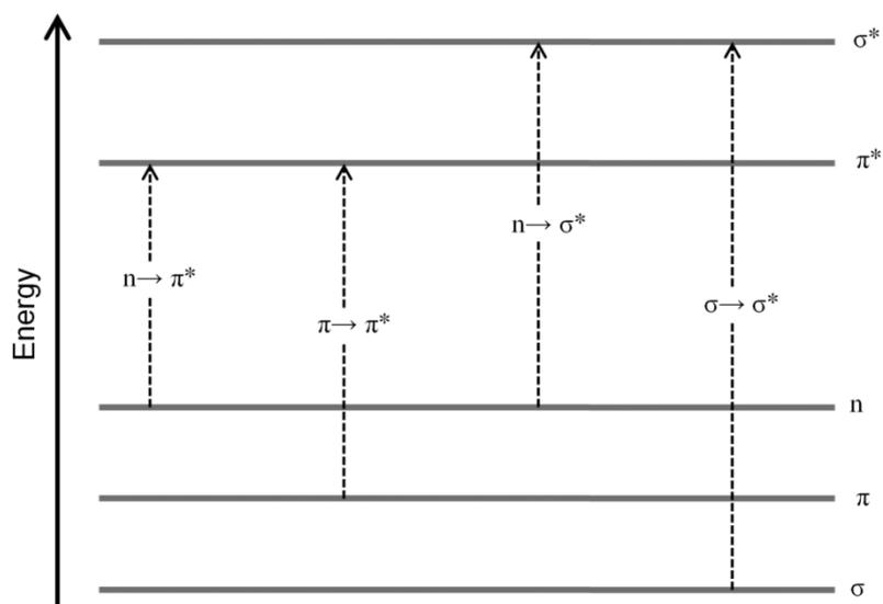
**Figure 4.1** A diagrammatic representation of the energy levels of molecular orbitals; the vertical arrows represent electronic transitions.
