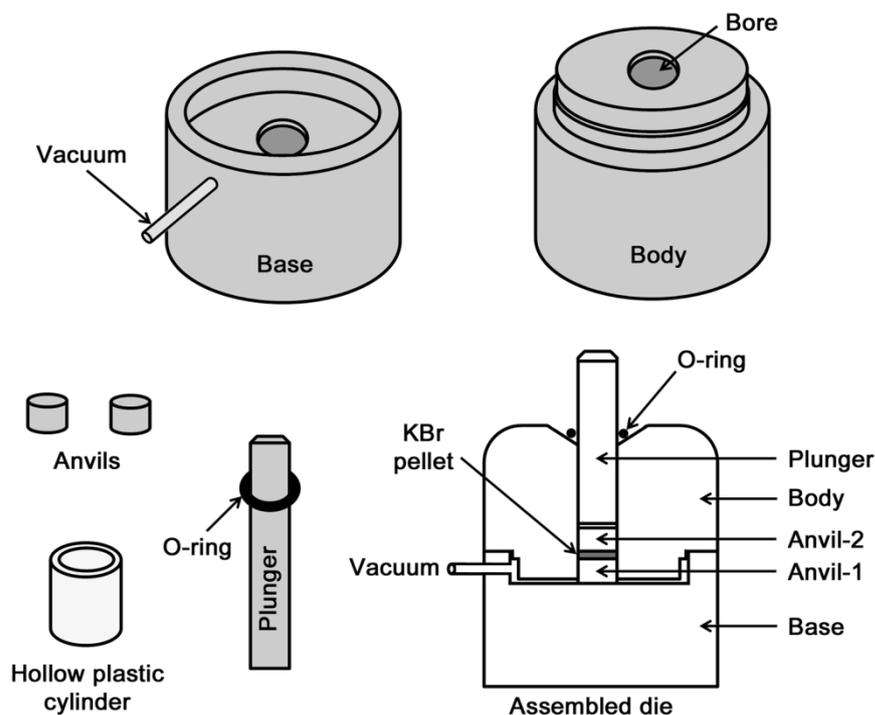
Figure 11.1: Different parts of a die for preparing KBr (and other) pellets
