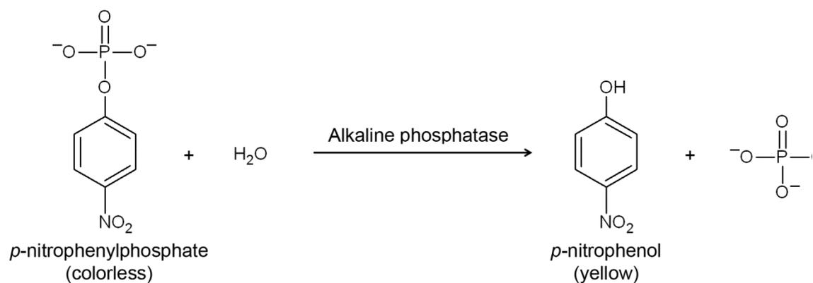
Figure 12.2: Hydrolysis of *p*-nitrophenylphosphate into *p*-nitrophenol and phosphate
