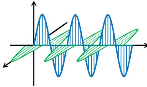
**Figure 9.1** Two plane polarized waves (blue and green), polarized in two perpendicular planes and out of phase by  $90^\circ$ . Only electric field vectors are shown here for clarity.
