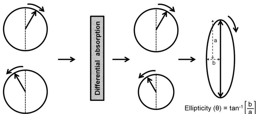
**Figure 9.3:**Differential absorption of left and right circular polarized light results in elliptically polarized light. Ellipticity is the arc tangent of the ratio of minor to major axis.
