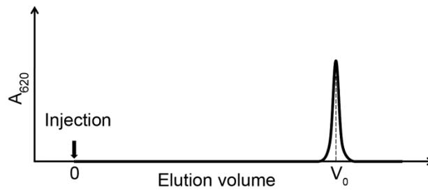
Figure 22.5: A chromatogram illustrating the void volume of a gel filtration column
