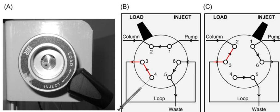
Figure 22.4: Injector valve (A); the diagram showing tube connectivities in load (panel B) and inject (panel C) mode
