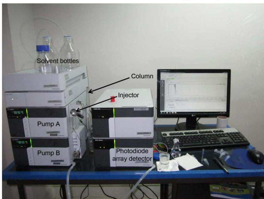
Figure 26.1: An HPLC instrument
