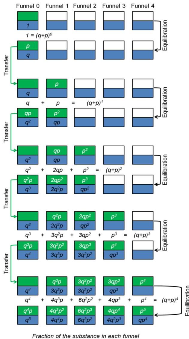
Figure 20.1 Distribution of a substance between stationary and mobile phases after transfers and equilibrations (please refer to text for details)
