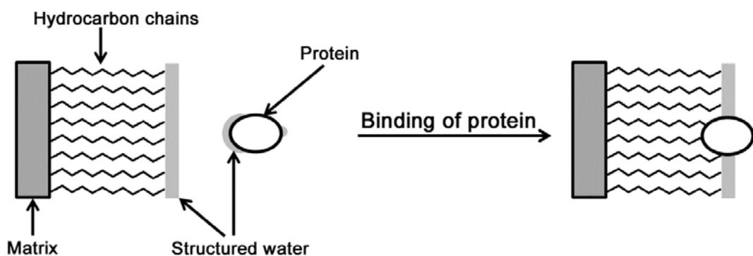
Figure 26.2: Interaction of a protein to a reversed-phase column; binding of hydrophobic regions of the protein to the hydrophobic stationary phase would displace the structured water molecules thereby increasing the entropy of the system.
