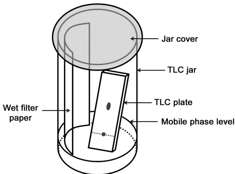
Figure 21.5: A thin layer chromatographic experiment set-up
