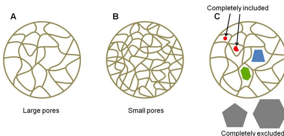
Figure 23.1 The diagrammatic representation of the beads with different porosities. Molecules completely included (shown in red) and completely excluded (shown in grey) are also shown in panel C.
