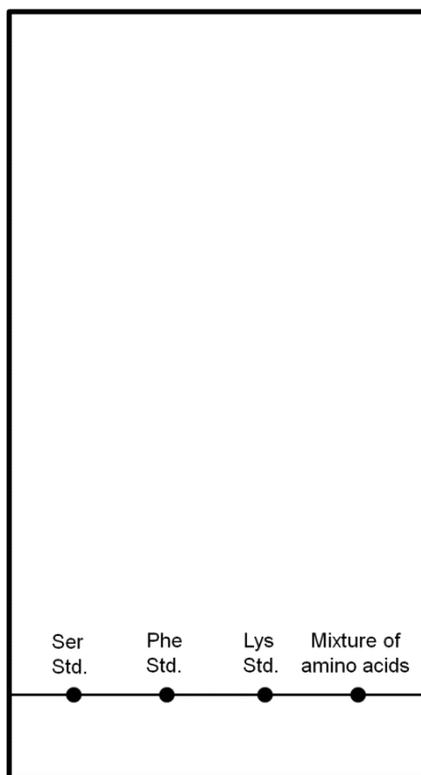
Figure 21.4: A thin layer chromatographic plate with spotted samples
