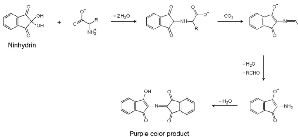
Figure 21.6: Reaction of ninhydrin with an  $\alpha$ -amino acid
