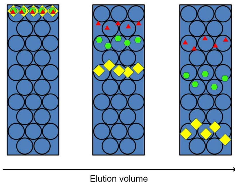
Figure 23.2: A diagram showing separation of molecules based on size in a gel filtration column
