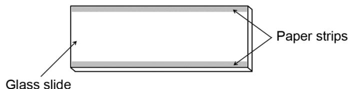
Figure 21.3: A diagram showing paper strips of equal dimensions placed along the long side of the glass slide
