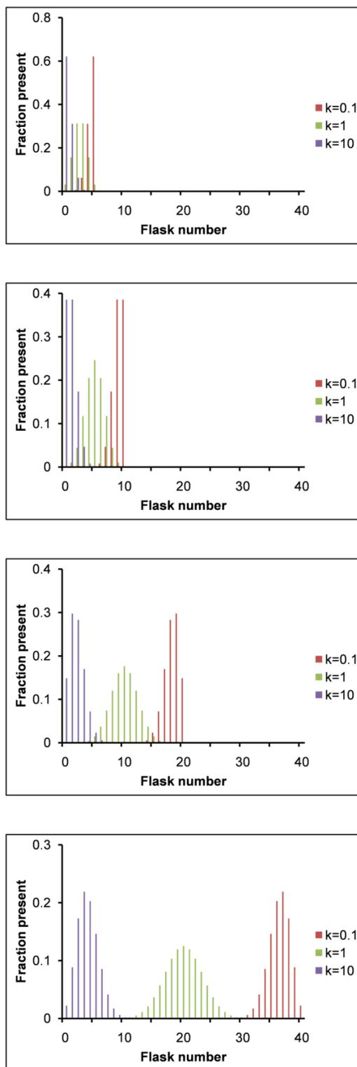
**Figure 20.2 Separation of three components having different partition coefficients for the two phases**
