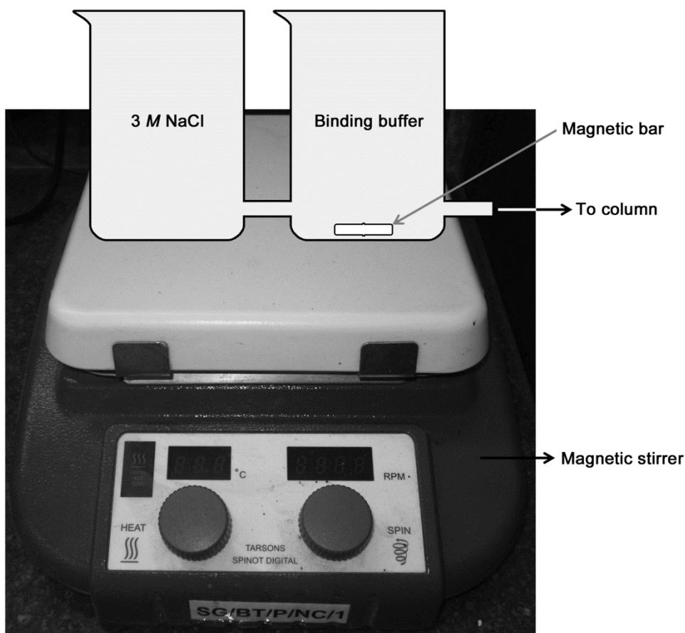
Figure 24.2: A gradient mixer kept on the magnetic stirrer
