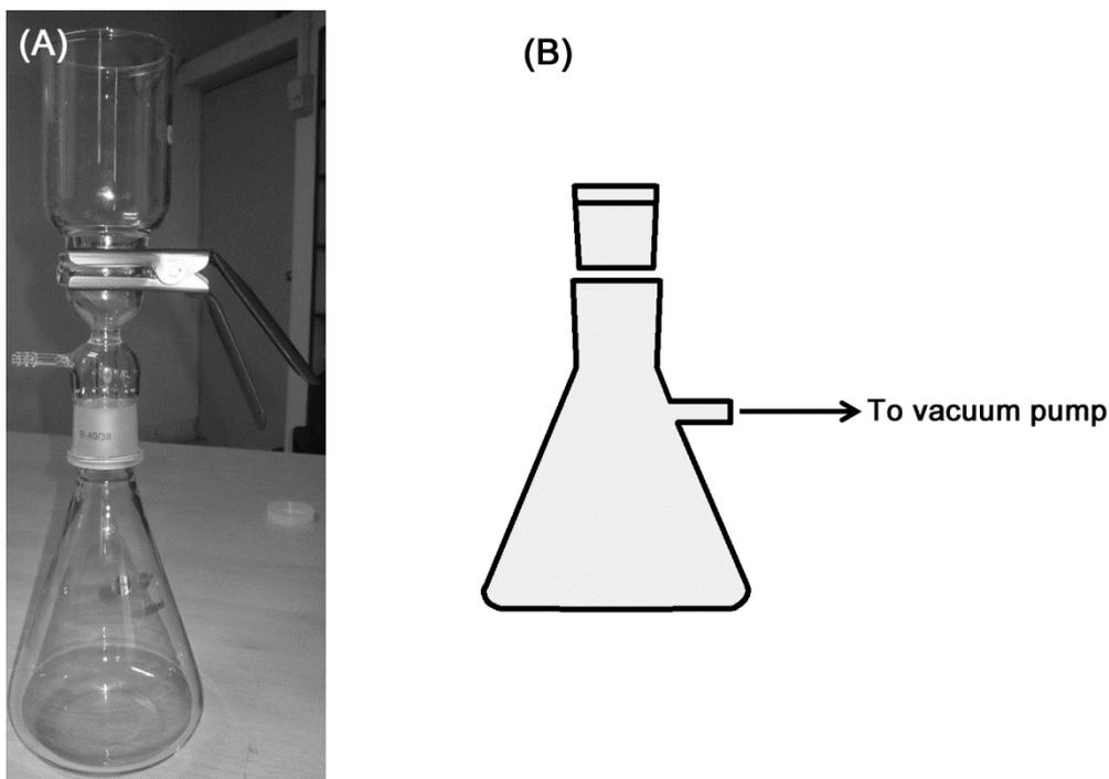
**Figure 22.1: A buffer filtration unit (panel A) and an Erlenmeyer flask for degassing (panel B)**
