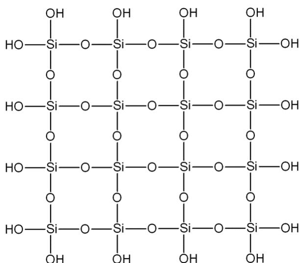
Figure 21.1: Structure of silica
